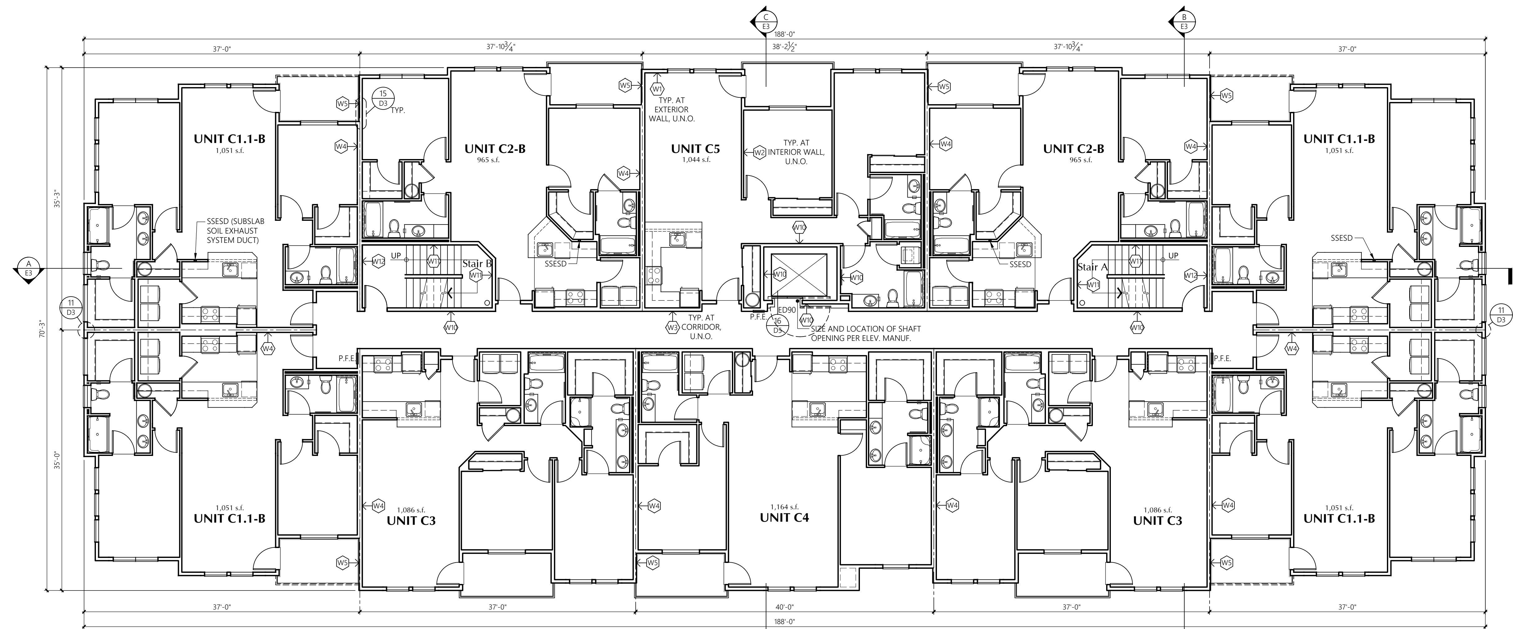
Building 3-6, 9 & 10 2ND FLOOR PLAN 1/8" = 1'-0"
